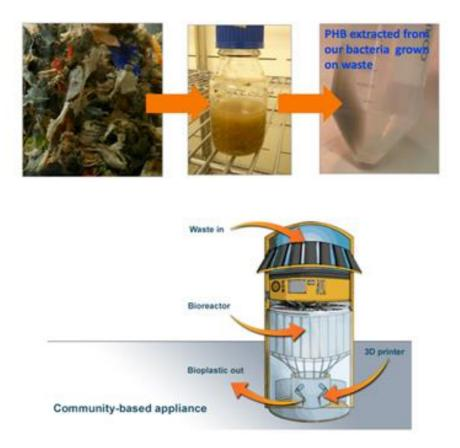
Figure 26. Plasticity: Production of bioplastics from non-recyclable waste.
