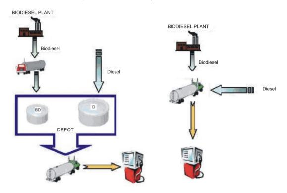
Figure 3.1.2.1: Biodiesel production chain
