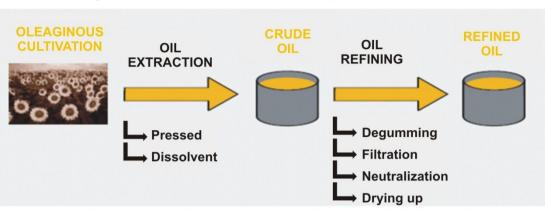
Figure 2.1.2.2: Outline of the productive process of refined oil
