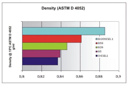
Graph 2.1.7.7: Density (ASTM D 4052) of the different mixtures
