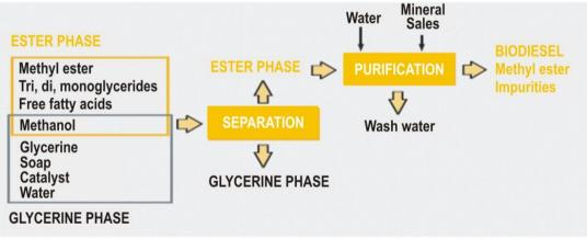
Figure 2.1.2.5: Outline of biodiesel's separation and purification processes
