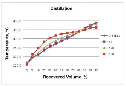
Graph 2.1.7.6: Distillation curve of the different mixtures
