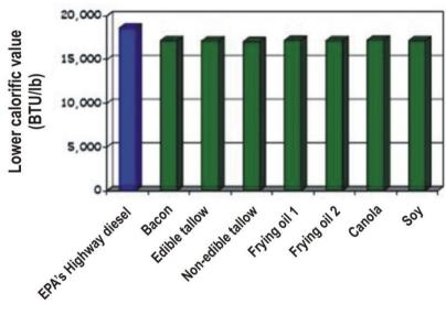
Graph 2.1.7.2: Energy content of diesel and different biodiesel
