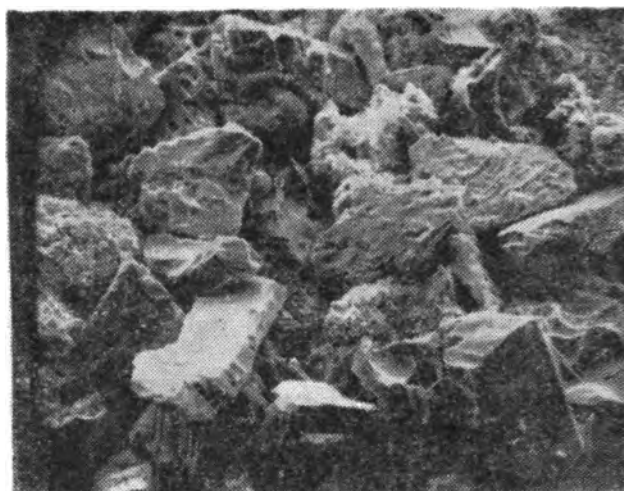
Fig. 3. Scanning electron micrograph (200X) of the very fine sand (.1-.05mm) fraction of horizon A1, profile 4.
